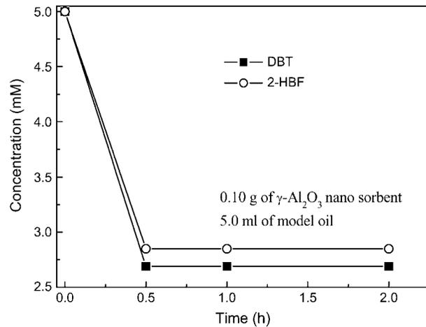
**FIGURE 3** Adsorption of DBT and 2-HBP using  $\gamma$ -Al<sub>2</sub>O<sub>3</sub> nanosorbents.
