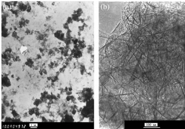
**FIGURE 1** TEM images of  $\gamma$ -Al<sub>2</sub>O<sub>3</sub> nanosorbent (obtained by Hitachi 8100, 200 kV). (a)  $\times 10,000$ ; (b)  $\times 200,000$ .
