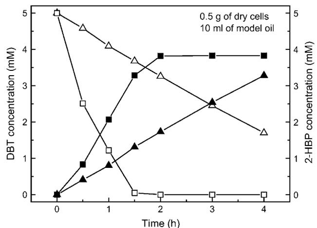
**FIGURE 4** Time course of desulfurization of DBT by free cells and  $\gamma$ -Al<sub>2</sub>O<sub>3</sub>-cells. Residual DBT concentration after being consumed by free cells ( $\Delta$ ); 2-HBP concentration produced by free cells ( $\blacktriangle$ ); residual DBT concentration after being consumed by  $\gamma$ -Al<sub>2</sub>O<sub>3</sub>-cells ( $\square$ ); 2-HBP concentration produced by  $\gamma$ -Al<sub>2</sub>O<sub>3</sub>-cells ( $\blacksquare$ ).
